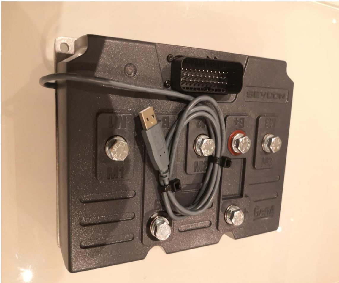
This is a modified Sevcon Gen4-48V-500A motor controller which is the same controller that was originally supplied on the Twizy 80. This will fit on all Twizy models like the Twizy 80 and Twizy 45 from 2012 to the present day. The controller has a built-in Powerbox Mini so here you get much more than a standard controller.
