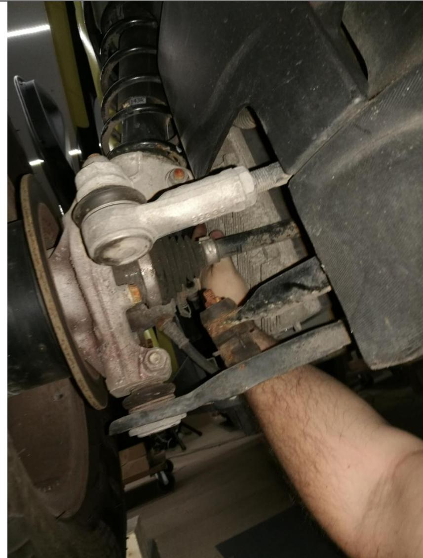
To gain access to the 2 screws at the top then slide your hand up on the outside of the controller heat sinks
