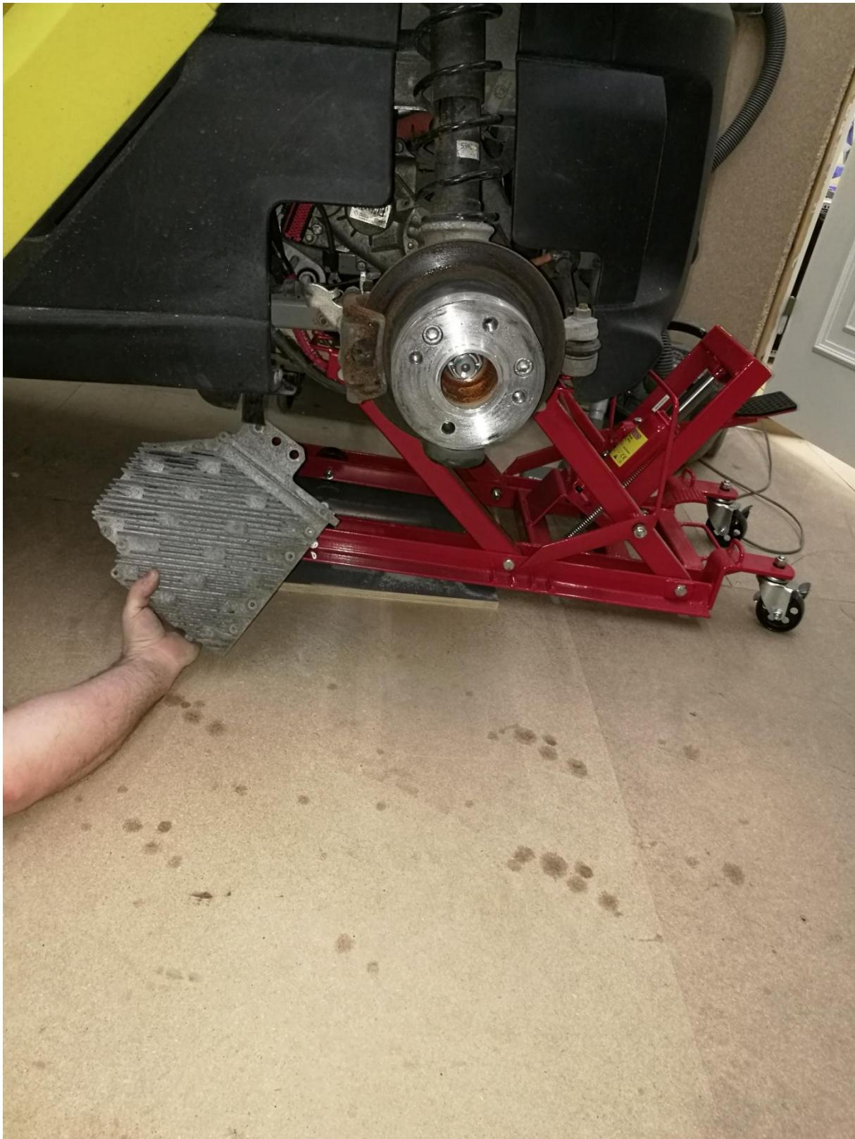
Now remove the heat sink and mount it on the new controller. Be a little careful about the orange gasket between the controller and the heat sink. If this gasket is bad you should buy a new one or use regular cooling paste. [Cooling paste](#) is the cheapest choice. (usually it goes without problems using the original gasket)
