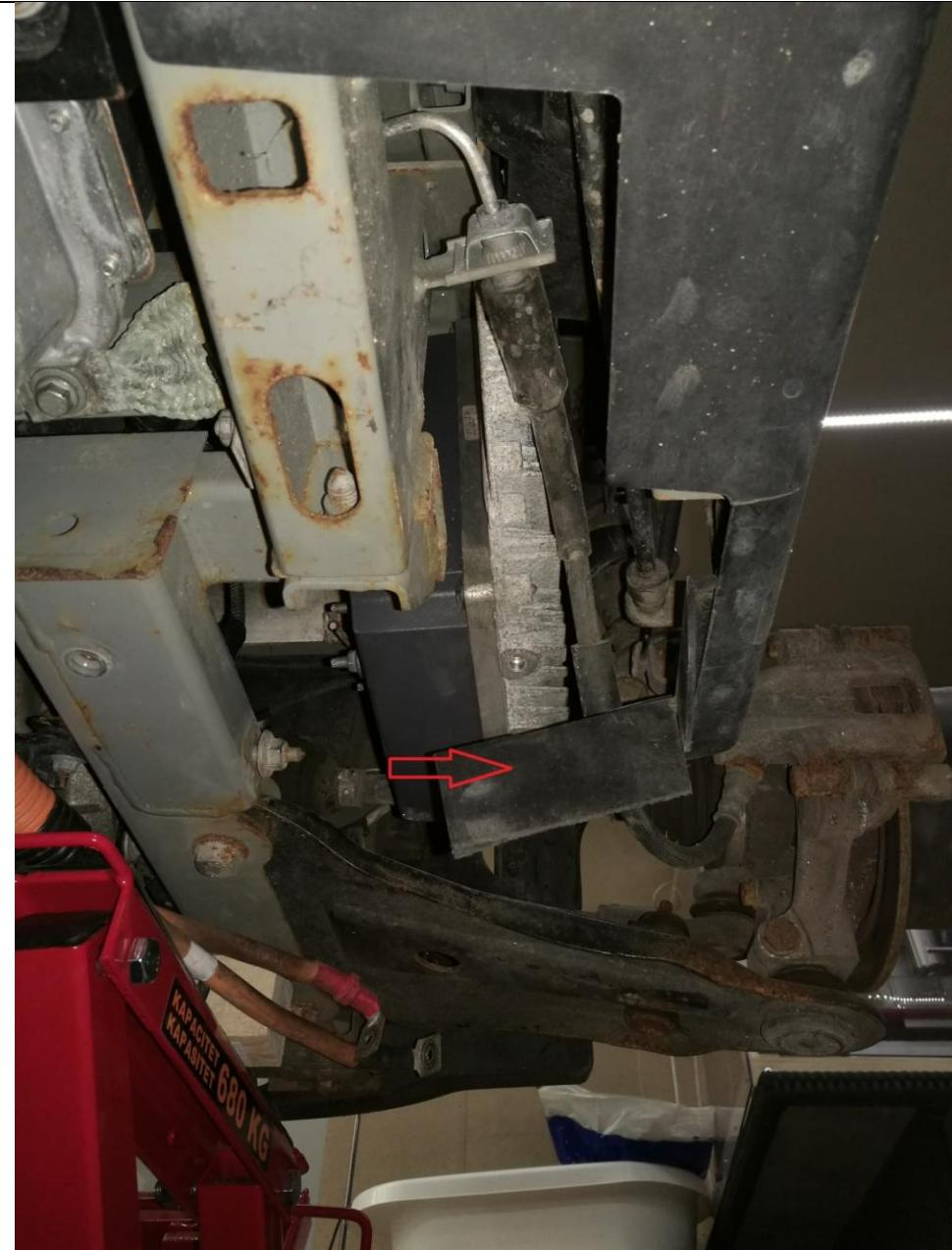
You can now remove the controller with sliding it downwards and slightly forward. bend away this plastic tap so you can get out the controller this way
